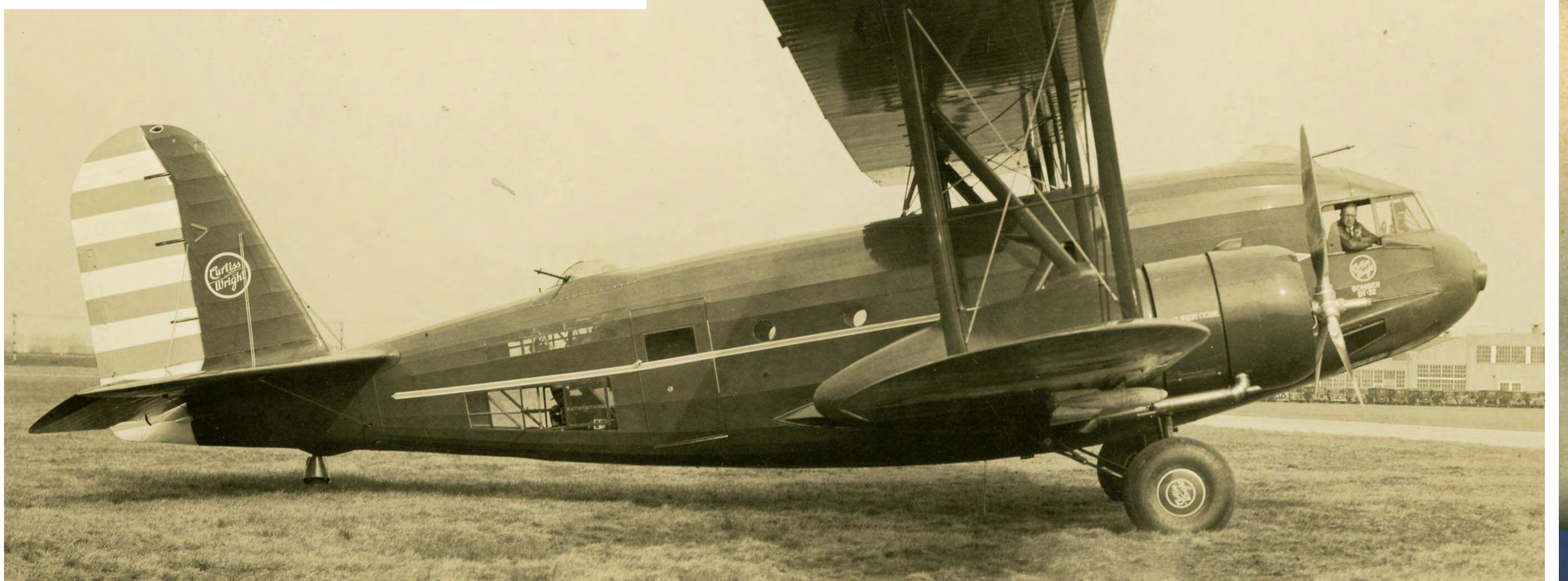
Curtiss-Wright Condor Bomber BT-32, a fifteen passenger plane powered by two Cyclone engines.
