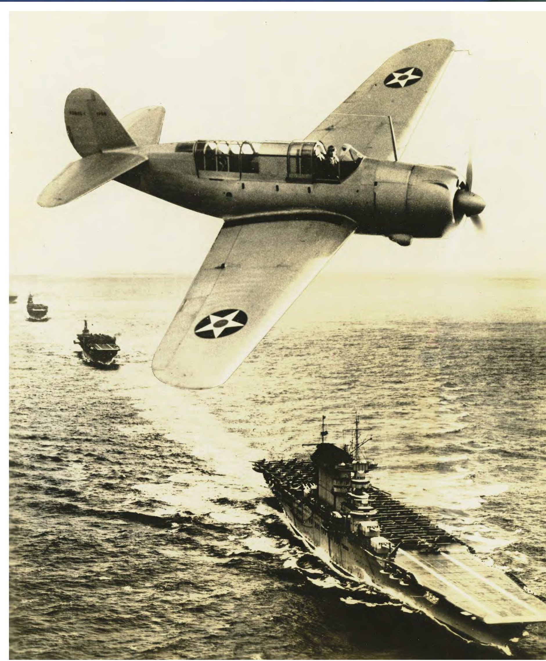
Curtiss SB2C-1 Helldiver, one of two hundred dive bombers made for the US Navy. Powered by an R-2600 twin Cyclone, 14 cylinder engine with a maximum speed of 295 miles an hour at 16,700 feet.
