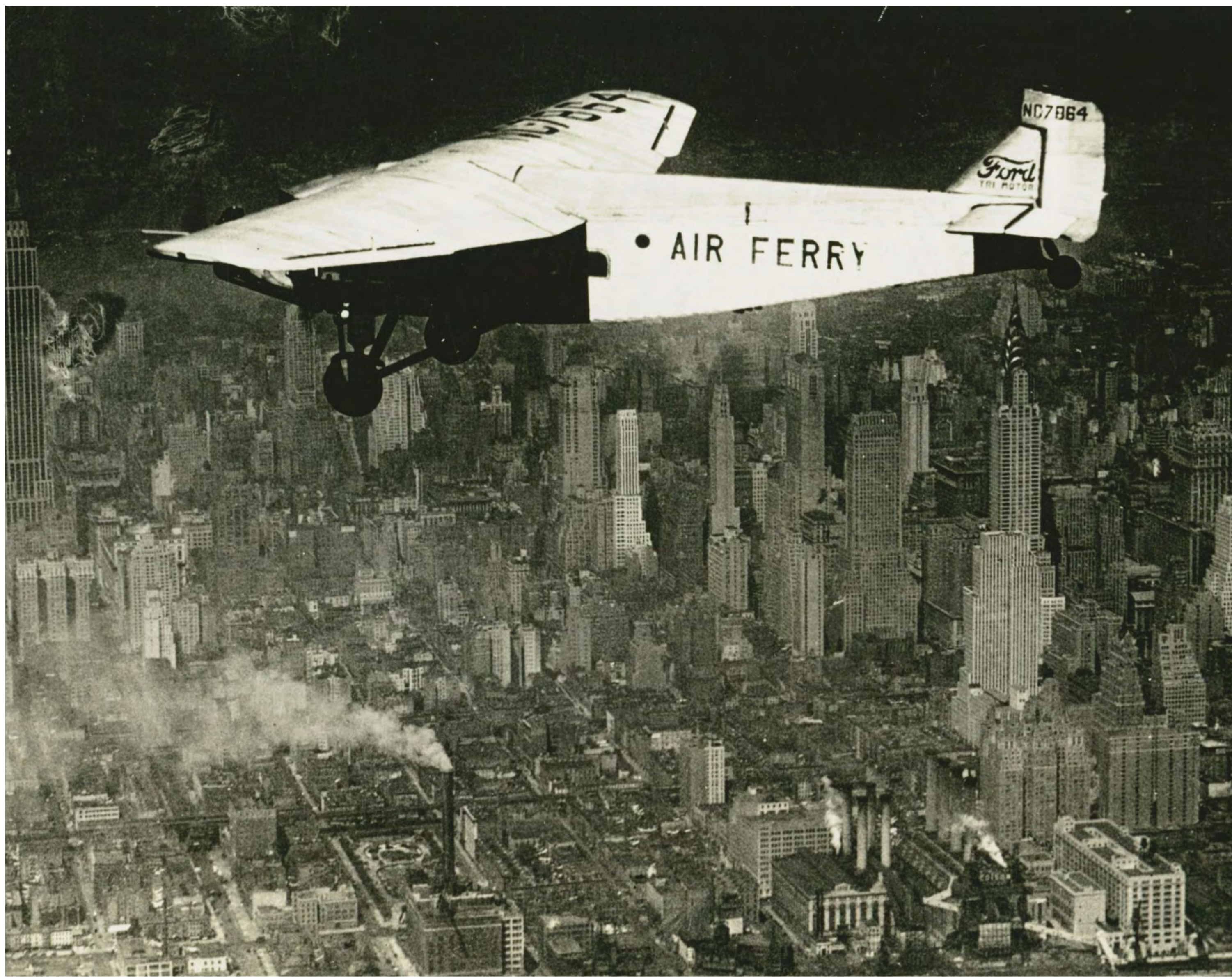
Air Ferry Ford Trimotor, powered by three Wright J-5 engines. Seen in flight over New York City, October 1931.
