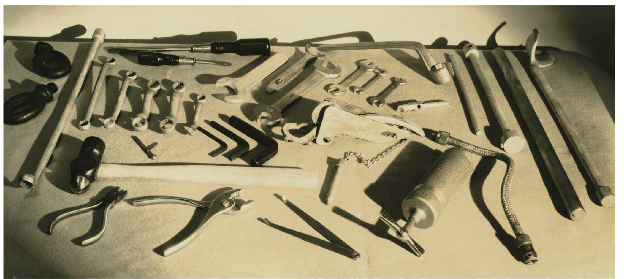
Wright Whirlwind engine toolkit, provided with each engine for maintenance.
