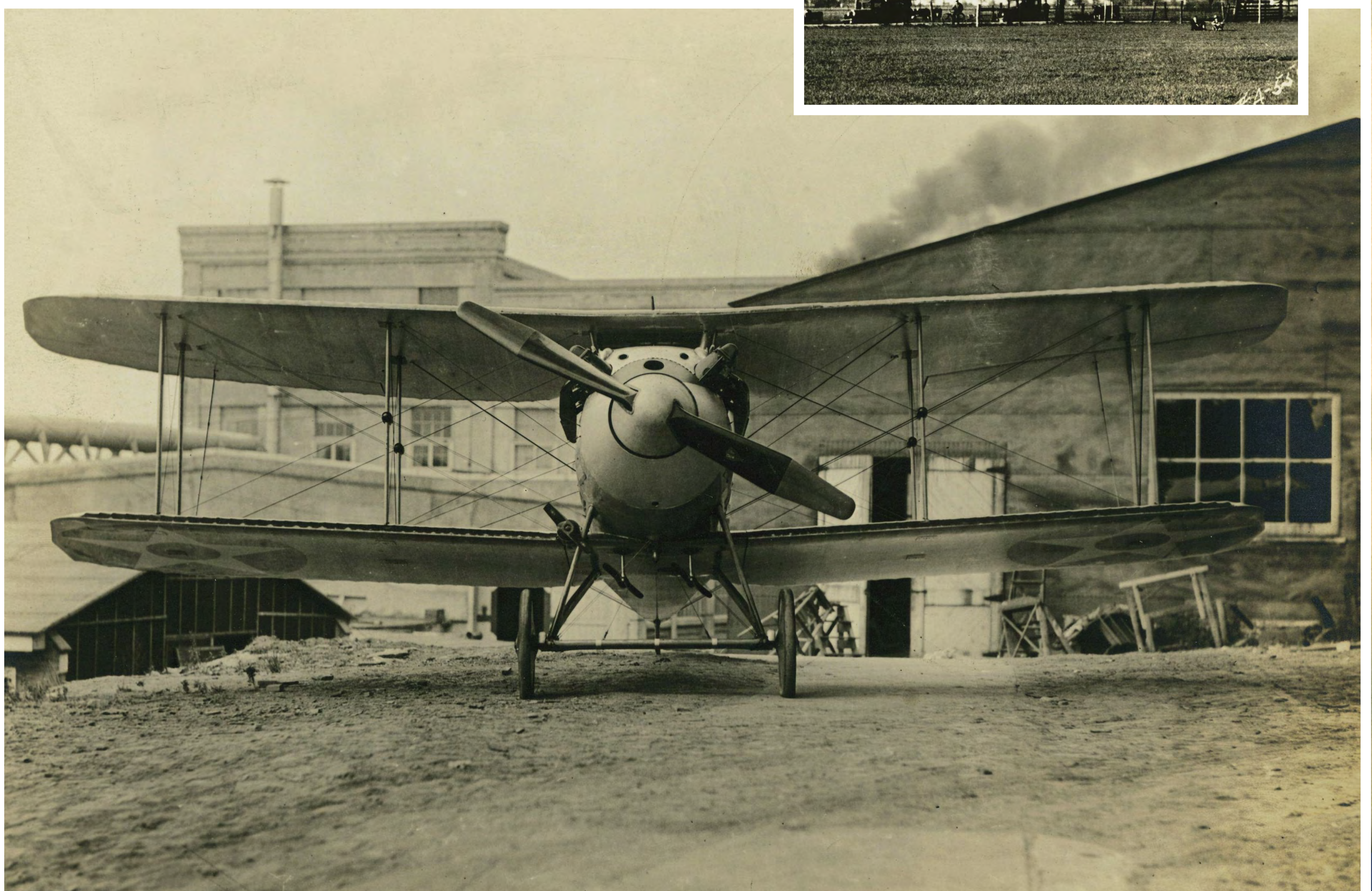
Thomas Morse MB-3 Pursuit Plane with a Hispano-Suiza engine (Wright V8 engine, 300 hp), 1919-1925.
