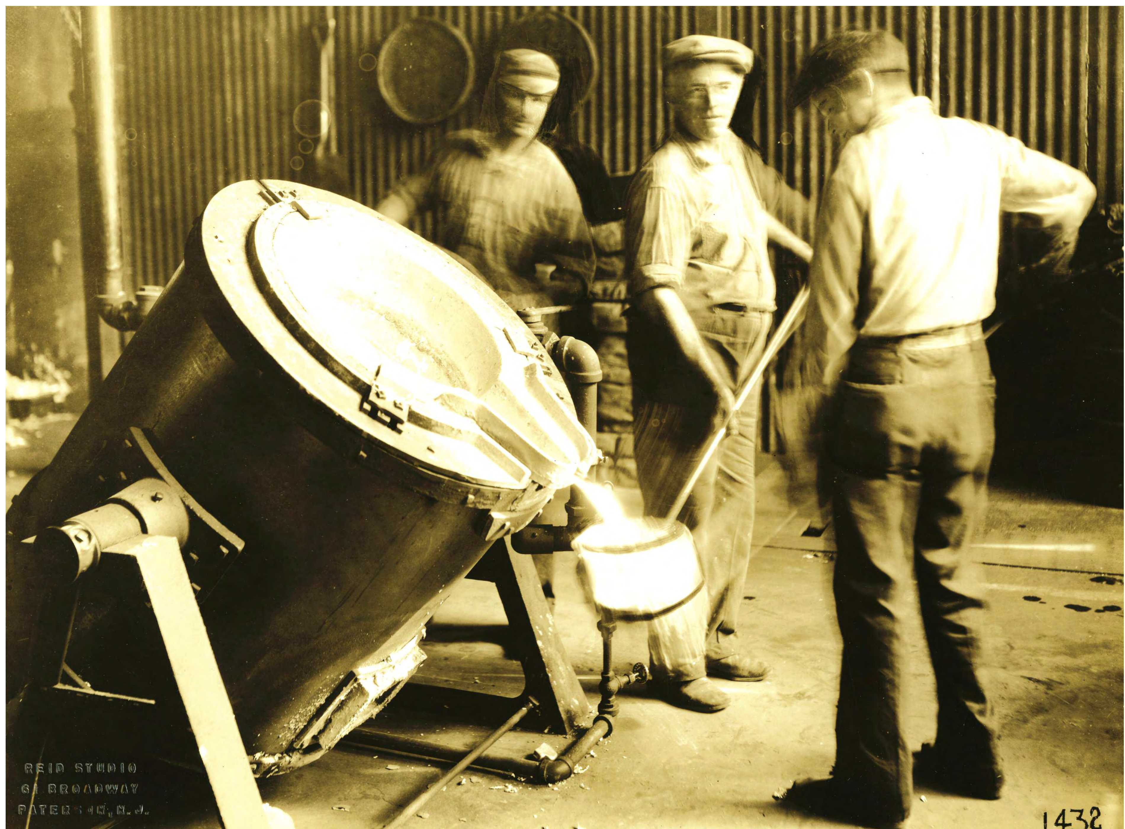
Foundry workers at Plant 1, pouring molten aluminum from a crucible into a smelting ladle or pouring pot. This metal was used in the casting of the engine's 8,000 parts.
