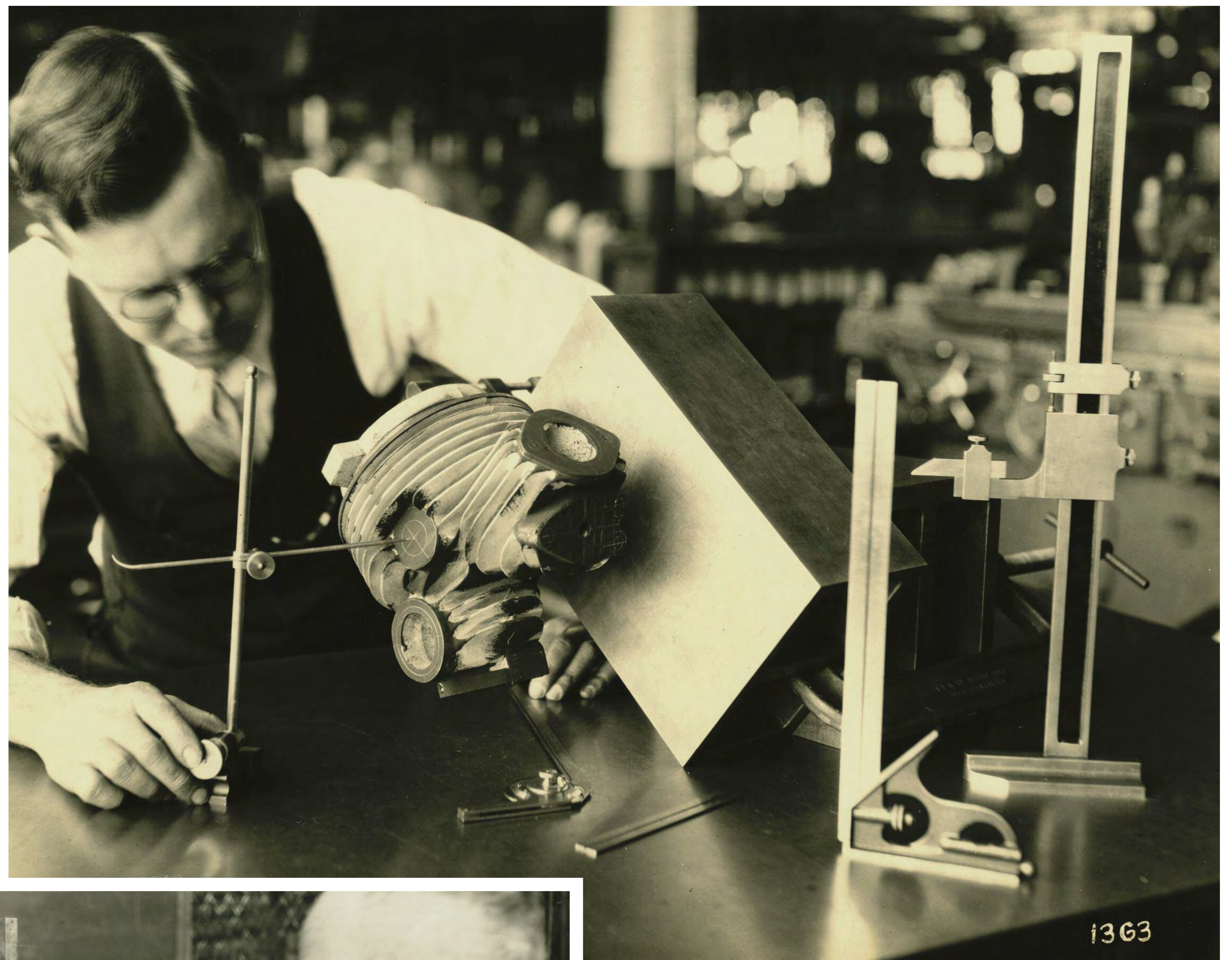
Laying out the intake and exhaust ports for drilling.
