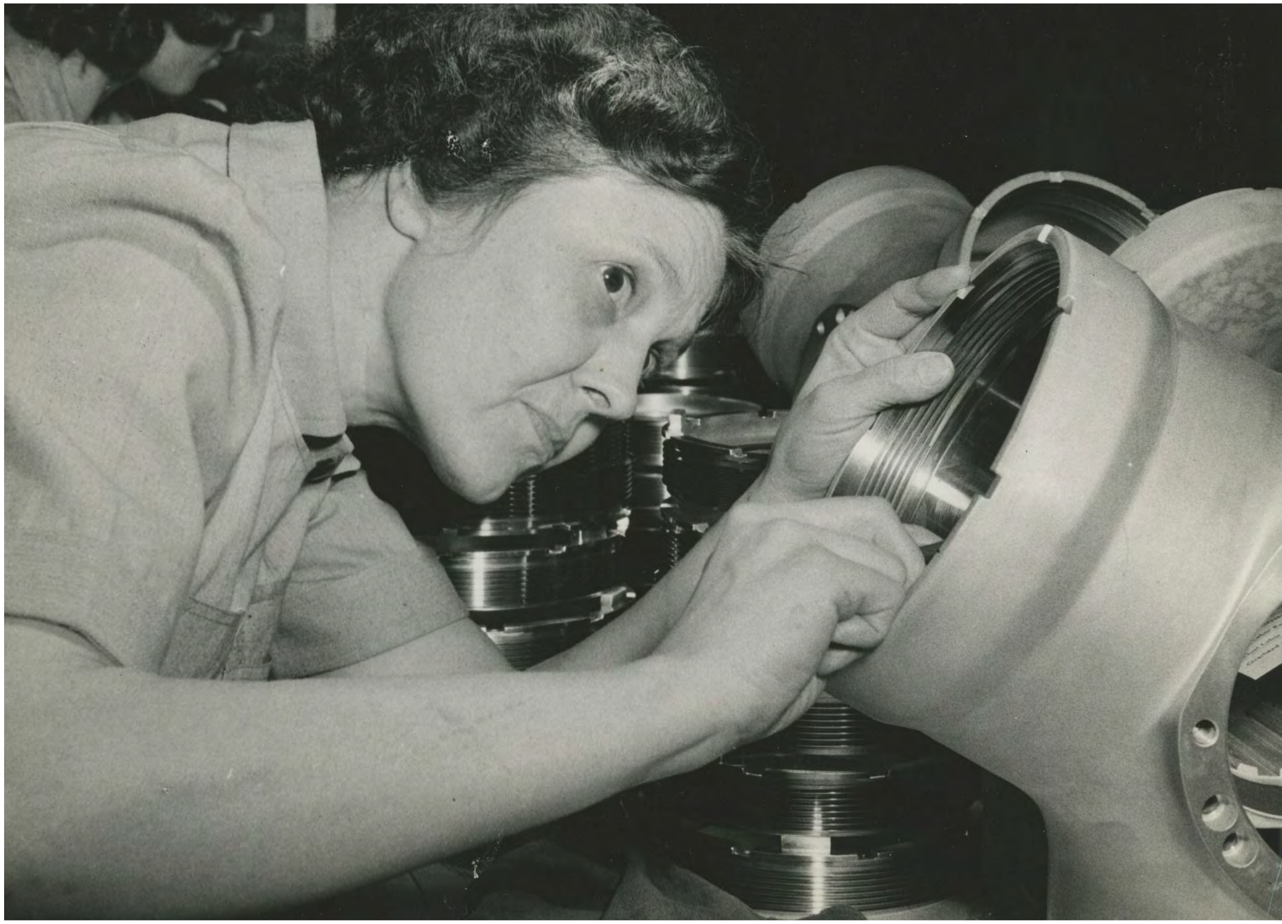
Mrs. Harriet Bruggess inserting threaded collars into propeller hubs for propeller attachment.
