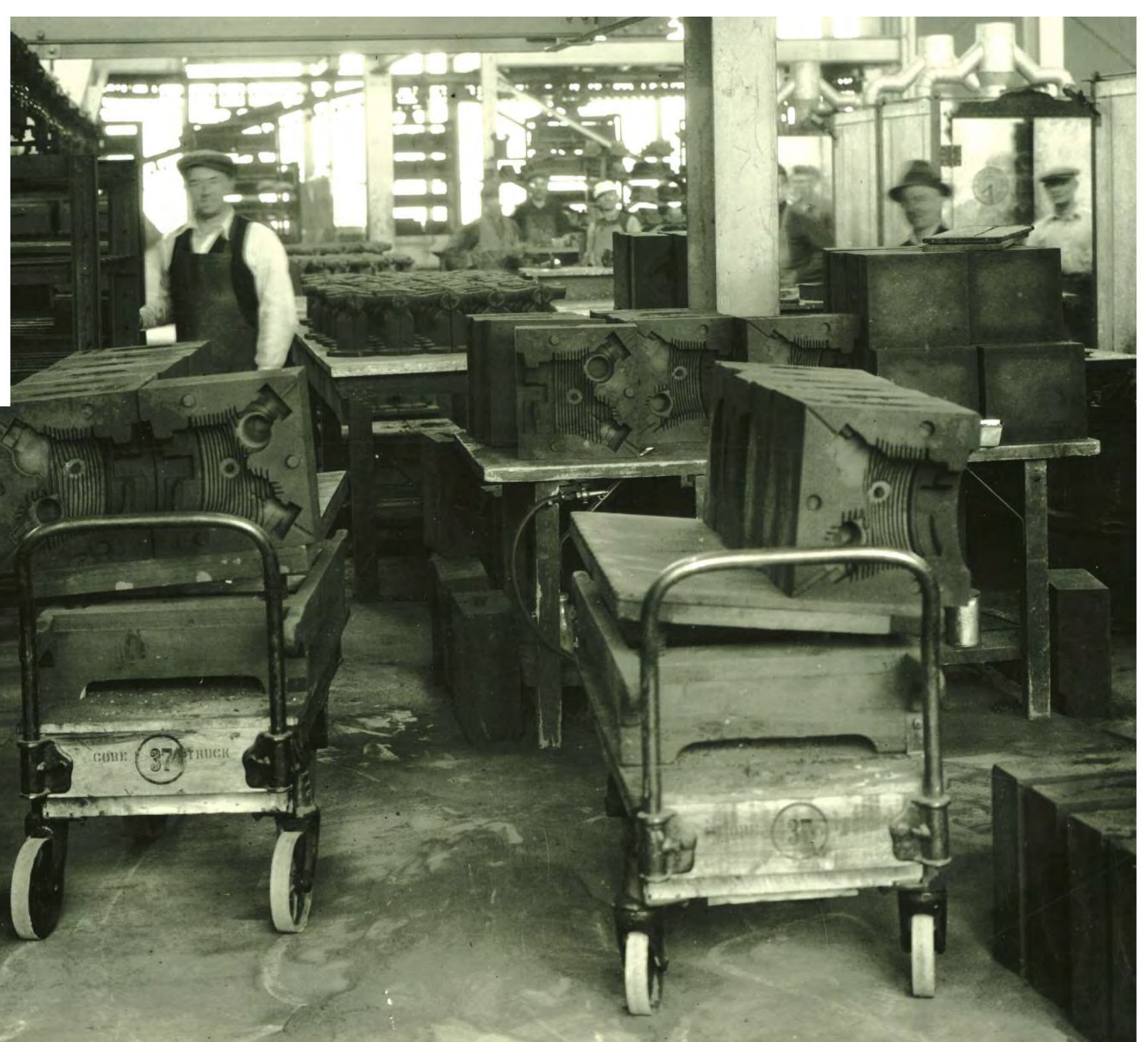
Prepared sand cast molds for cylinder heads, waiting to be transported to the foundry for casting.
