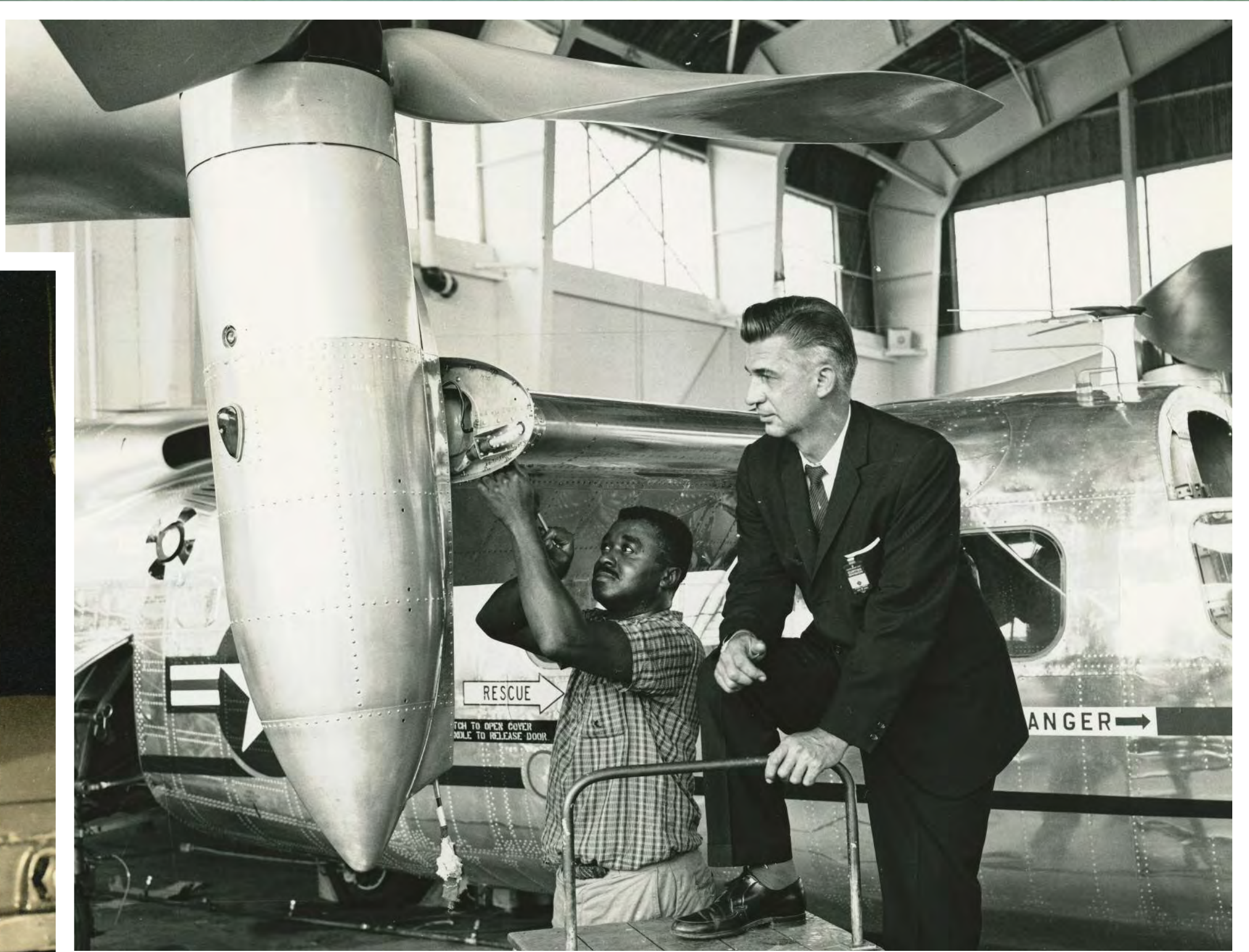
Making adjustments to the Curtiss-Wright X-19 VTOL (Vertical Take-off and Landing) circa 1960.
