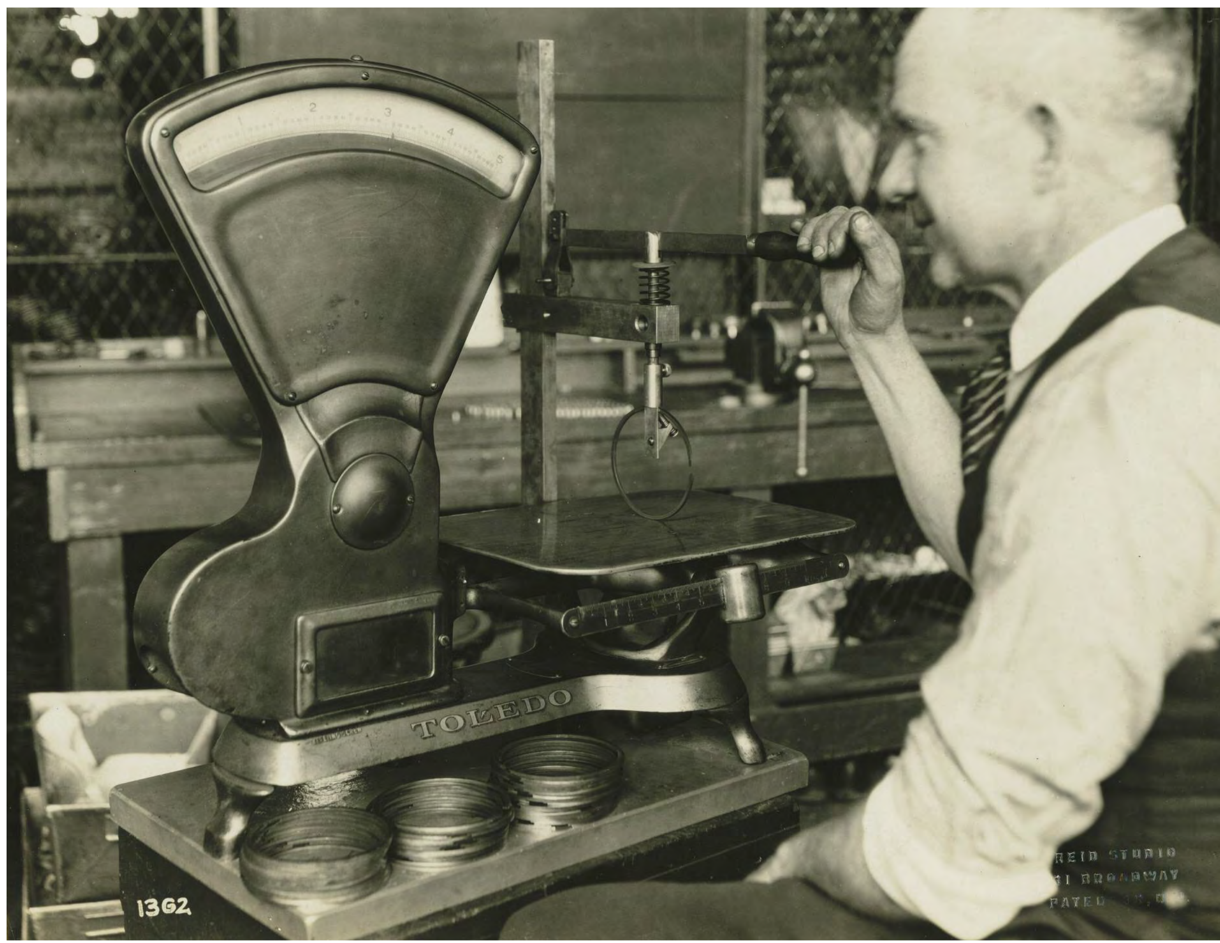
Testing the compression of a cylinder ring.
