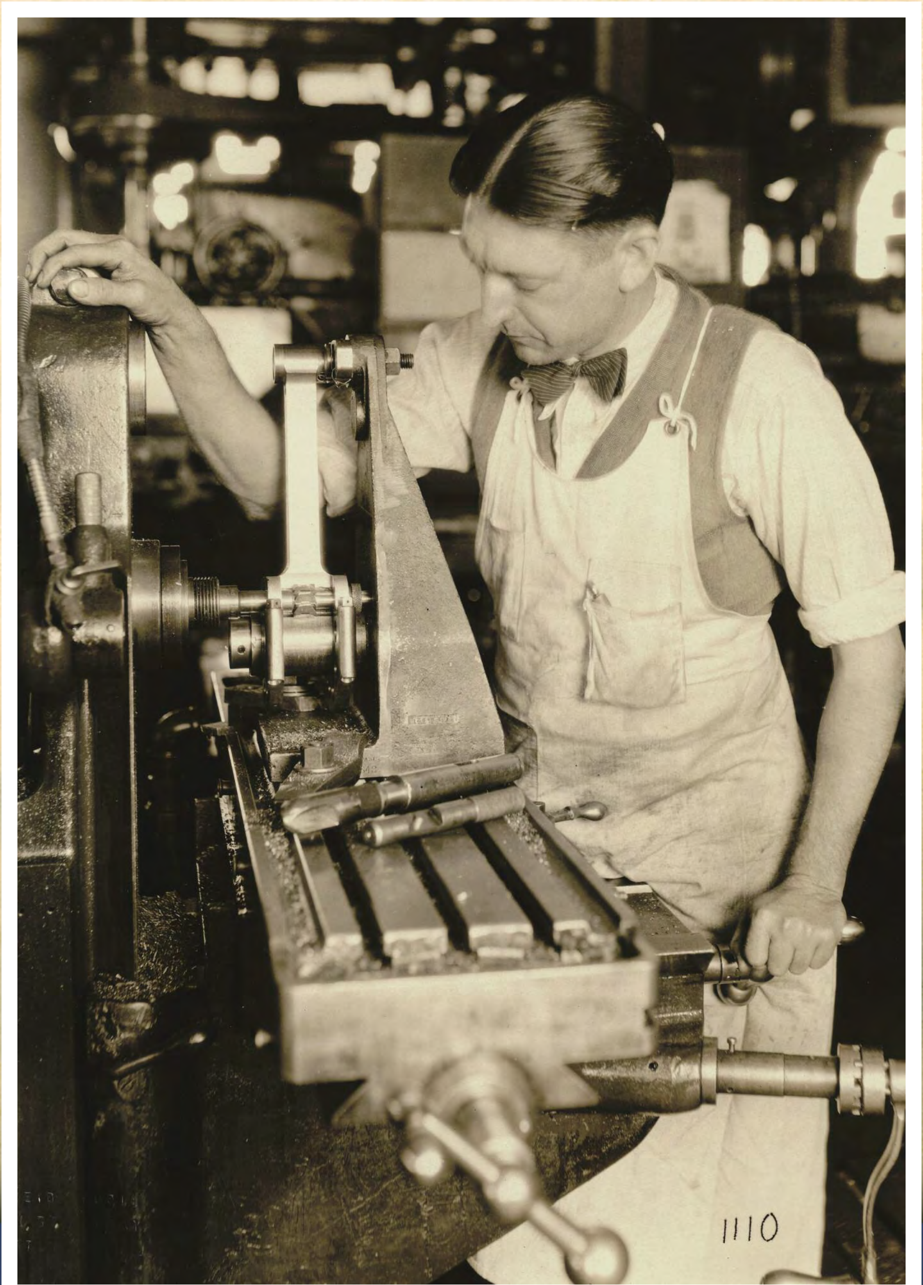
Using a horizontal mill to drill a clearance in the master rod for placement of the articulated rod knuckle pin.
