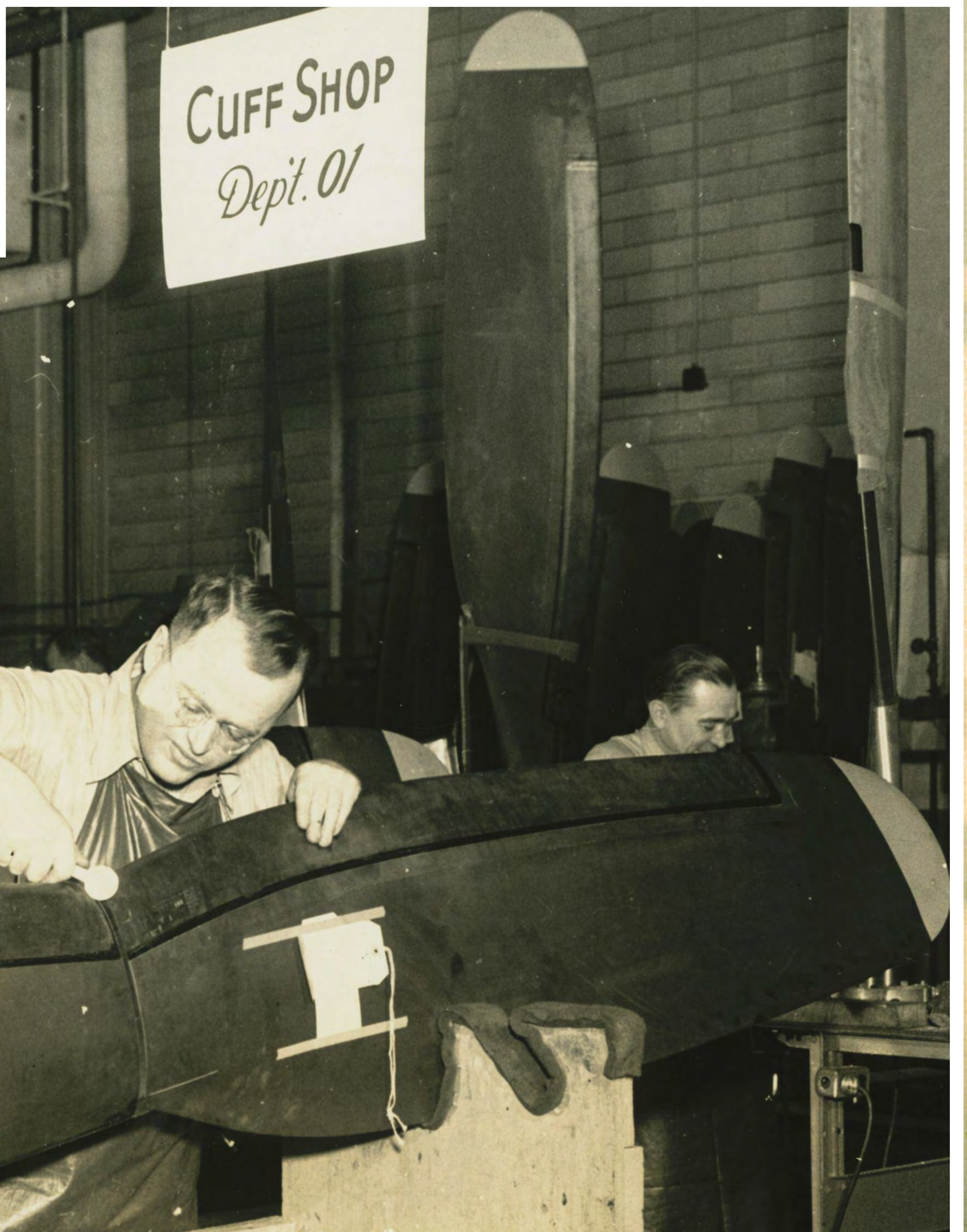
Line assembly techniques were employed to speed output of propeller blade electrical de-icing systems. Curtiss-Wright Corp. factory, Caldwell, NJ, August 22, 1947.
