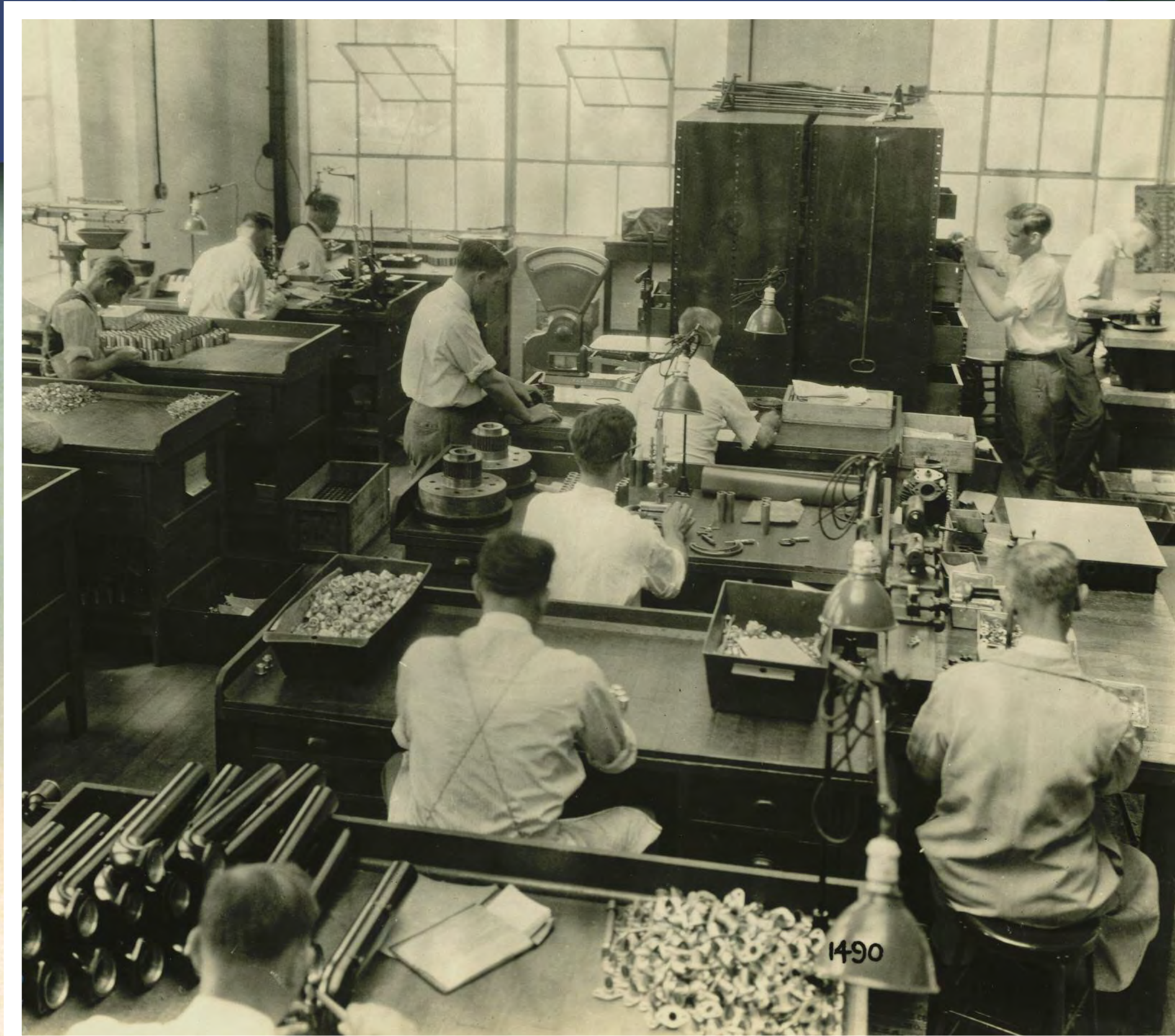
Employees inspecting various components. Over 50,000 tests were conducted per engine in the course of manufacture.
